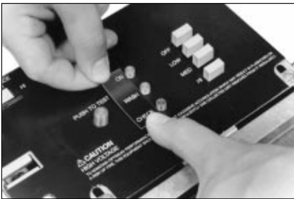
5. ATTACH NEW STICKER TO SWITCH COVER ASSEMBLY.
