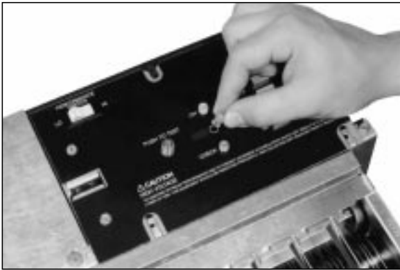
3. PUSH LED LENS INTO PLACE.
